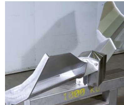
Detail view of the pre-masher (left picture)
