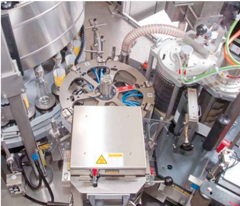
Labelling station with replaceable hotmelt gluing unit
