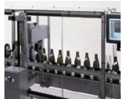
The machine guard of the Checkmat 707 F-X with x-ray measuring technology complies with the DIN EN 294.
