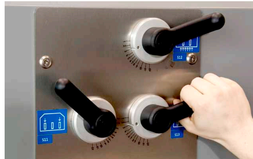
Easy adjustment of the air nozzles
