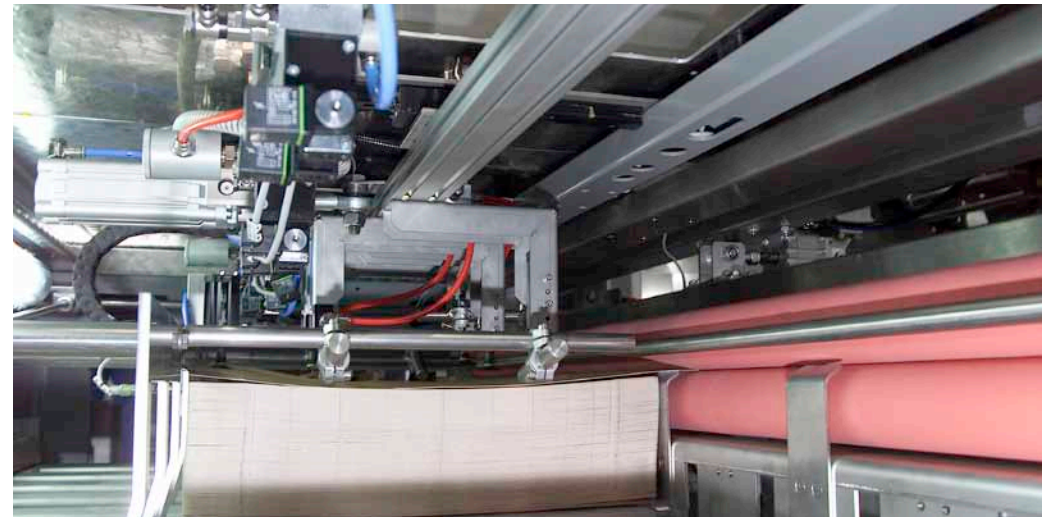
Roller separator feeding the separated cartons.
