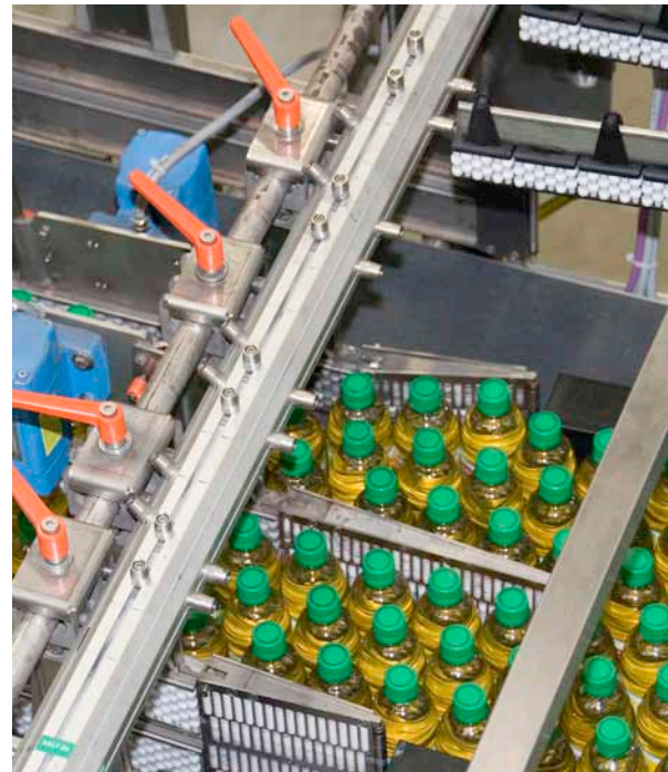
Variable lanes at machine infeed
