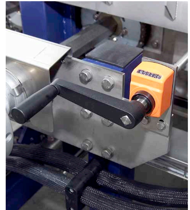
Crank for infinite adjustments
