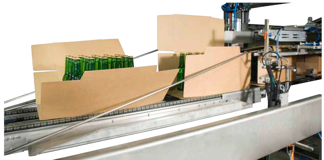
Guide bars unfolding the carton.
